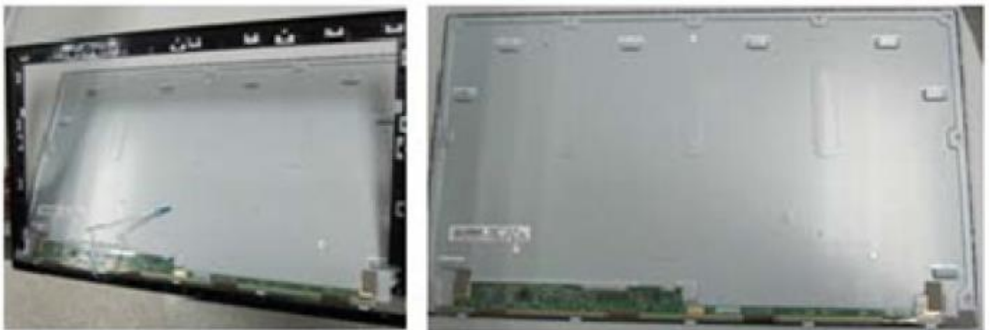
Step.9 Remove from MID frame
