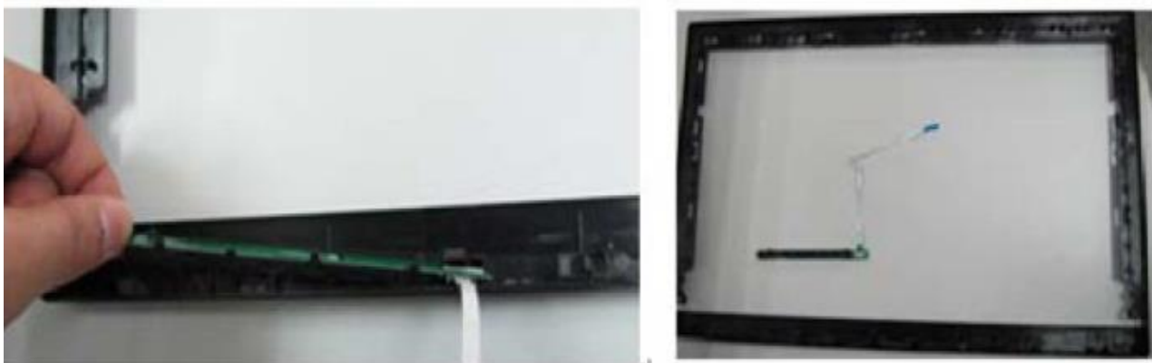
Step.11 Separation the cable and the plastic
