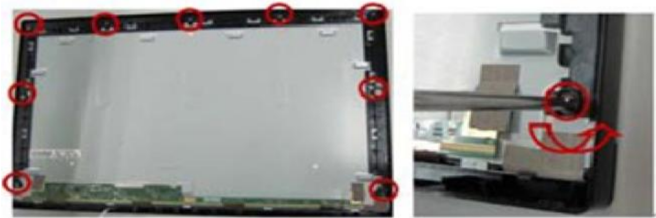
Step.9 Remove from MID frame
